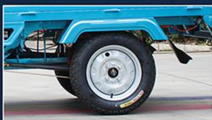
Steel wire tire: Front 350-12, Rear R400-12
