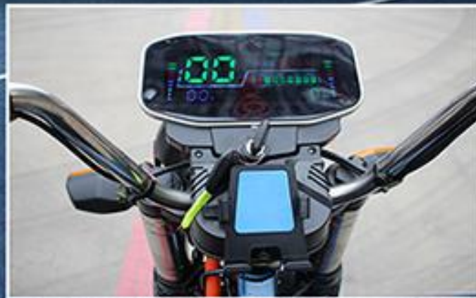
The LED digital instrument panel provides intuitive data and bluetooth connectivity
