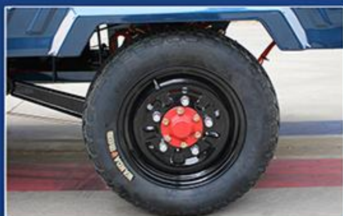
High-strength steel wire tires offer superior grip. Tire: Front 375-12, Rear 400-12
